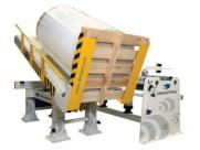
Central unwinding system with a 3"steel expansion shaft.
